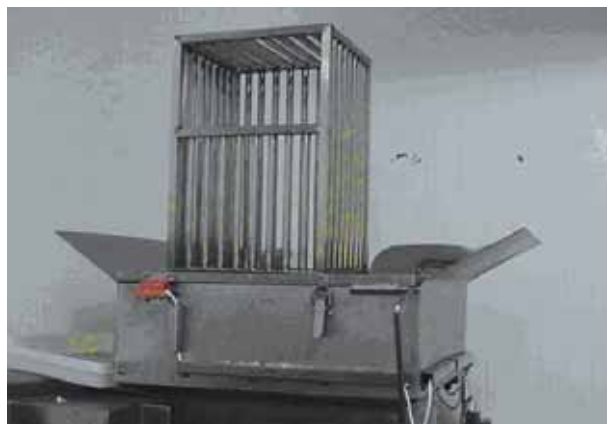
Above an interlocked extended reach guard for hand feeding
