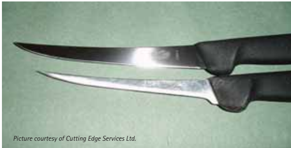
Figure 2: a knife worn to the point where it would be unsafe to use
